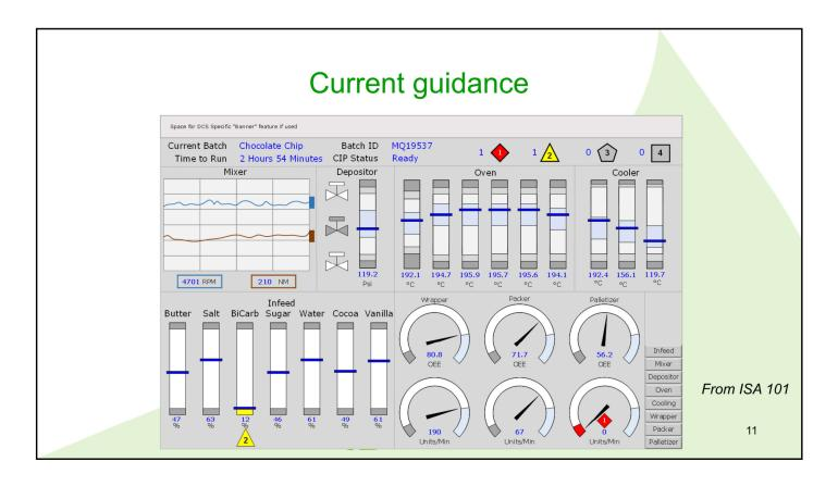
This is an example of some recent guidance for developing overview graphics for control room operators. It moves on from the previous historical examples I showed a minute ago and uses some of the display principles from the previous slide. Whether operators like this and find it useful is still to be confirmed.
