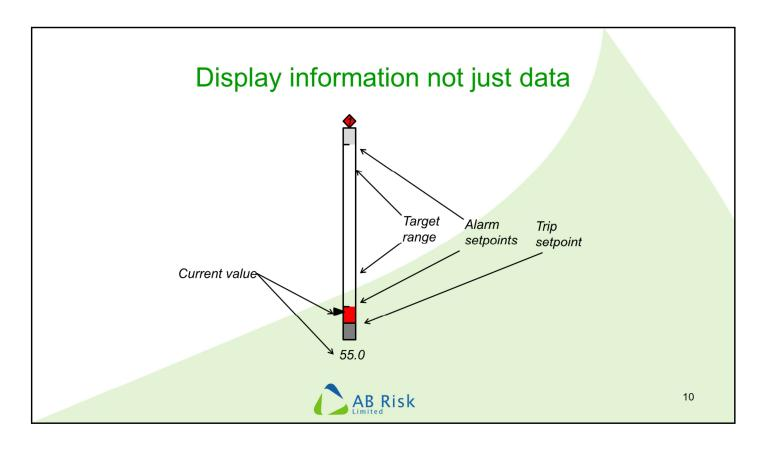
This image shows how a graphical representation can gives better situational awareness than a number showing the current value for a variable. From a very quick glance the operator can quickly understand how the plant is doing in relation to the measured range and target values. Colour and the graphical symbol at the top alert them in this case to the variable being in alarm.
