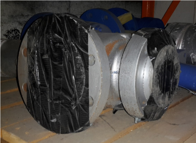
Figure 3: Example of a PSV with flanges covered in tape and stored on its side
