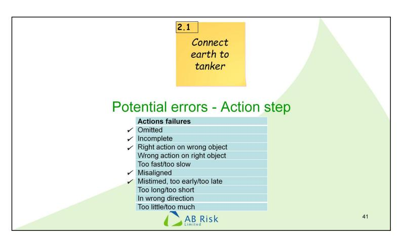
We then consider which errors on this list could happen. As you can see we have rejected some of the possibilities because we could not see how they could occur given the design of the earthing connection used.
