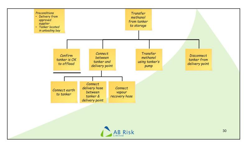
The next stage is to start adding the details in the form of task steps. The same rules apply about the number of steps in that you are aiming for less than 10 for each, if possible. Not a hard and fast rule but an important guide.
