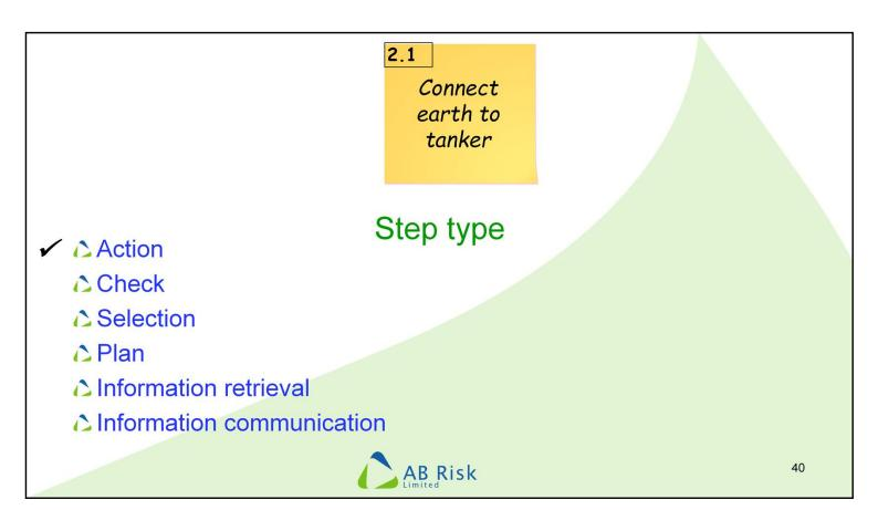
If we look at the step of connecting the earth to the tanker. If you don't know, this is intended to stop static electricity from building up because the spark it causes could start a fire.
