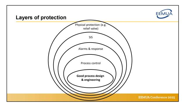
The introduction of more sophisticated automatic control and Safety Instrumented Systems (SIS) seems to lead us to safer systems. But event this traditional representation of layers of protection shows that there is a critical role for the human to accept and respond to alarms. Why would we do that if humans are so unreliable? The answer is that we have created systems that don't want to run. We need people to stop the SIS activating.
